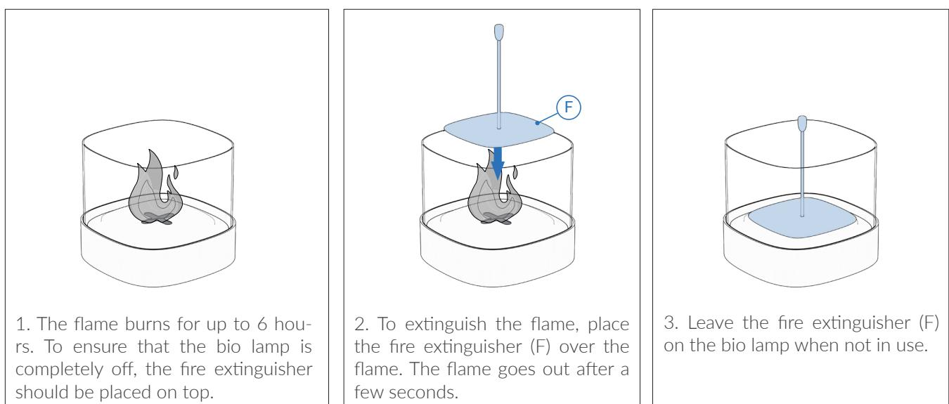
1. The flame burns for up to 6 hours. To ensure that the bio lamp is completely off, the fire extinguisher should be placed on top.
