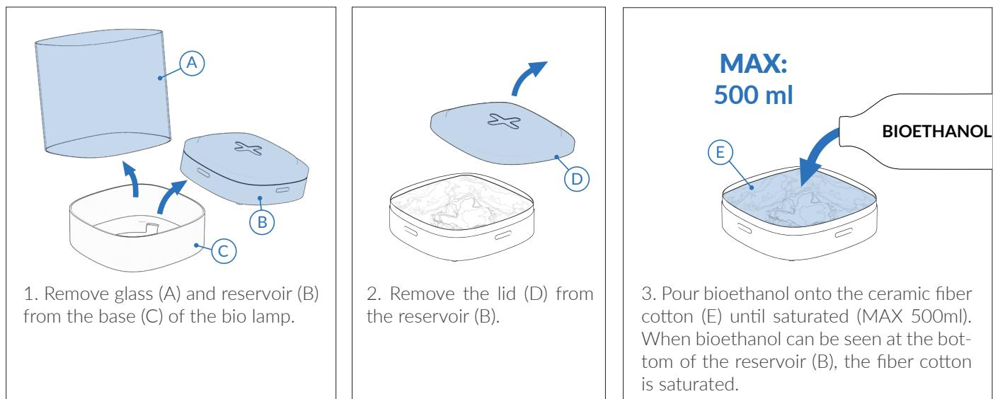
**NOTE:** Never overfill the reservoir! Do not fill the reservoir to the edge with bioethanol. When there is more bioethanol in the reservoir than the ceramic fiber cotton can absorb, it can easily overflow while handling the bio lamp and it can burn uncontrollable. The ceramic fiber cotton must remain in the reservoir and may only be removed when replacing it.
