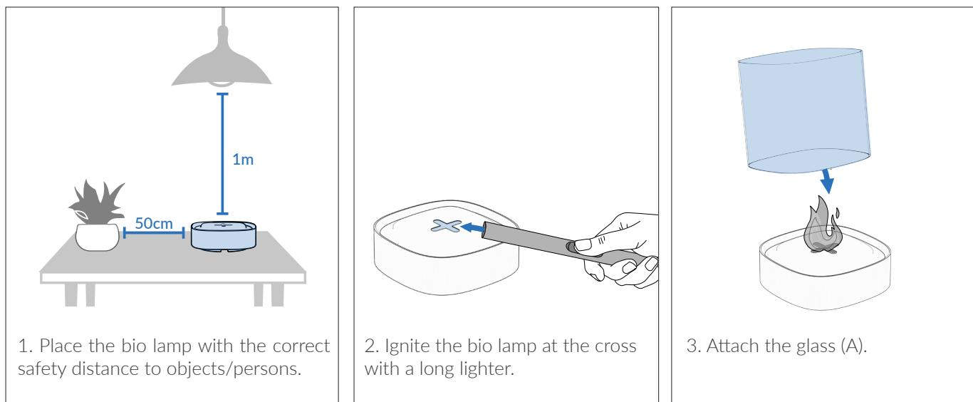
**NOTE:** Avoid holding your head over the bio lamp during ignition. Keep hair and loose clothing away from the bio lamp when it is lit.
